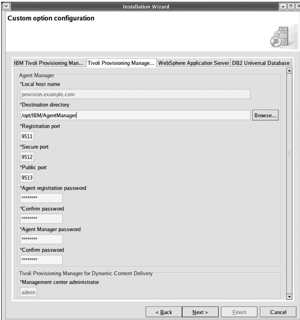
Figure 12. Tivoli Provisioning Manager components configuration
